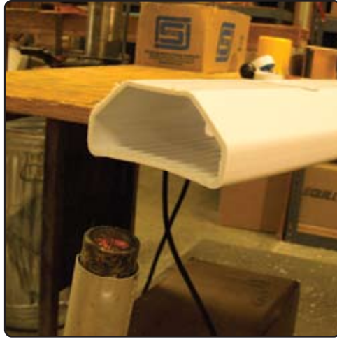
Heat Bottom of channel
